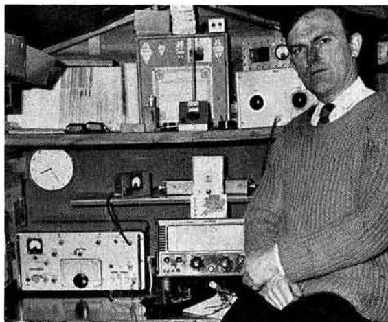
Photo of the author taken in 1967 at a previous QTH in Luton. Layout shows swr meter, low-pass filter, atu and screened dummy load
